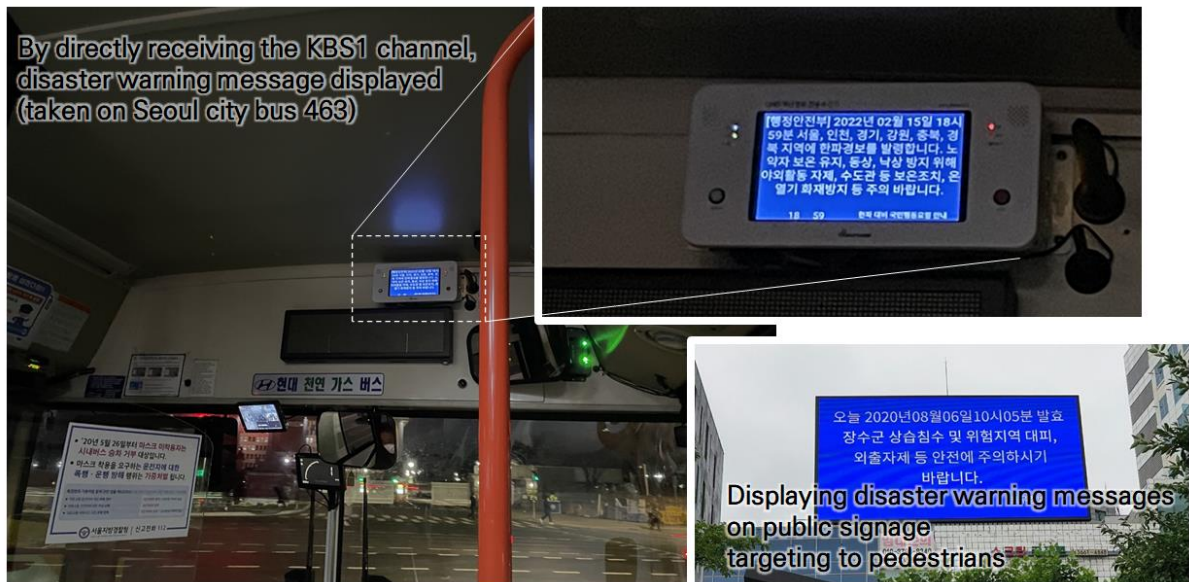
Figure 2.2.2 Disaster warning message displayed on a special receiver installed in Seoul city bus and public signage on the street equipped with ATSC 3.0 direct reception function
