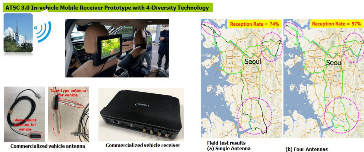
Figure 2.2.3 (left) An ATSC 3.0 vehicle receiver prototype capable of mobile reception with up to 4 antennas Diversity (right) Field test results of mobile reception success rate in Seoul metropolitan area when one or four reception antennas are used
